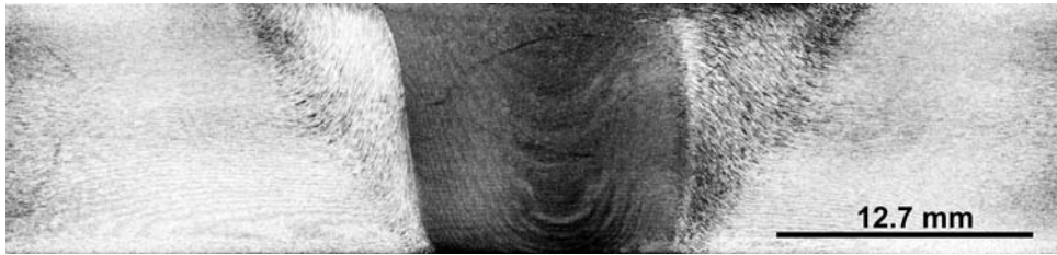
Fig. 3 Metallographic cross section of 7075 friction stir weld
